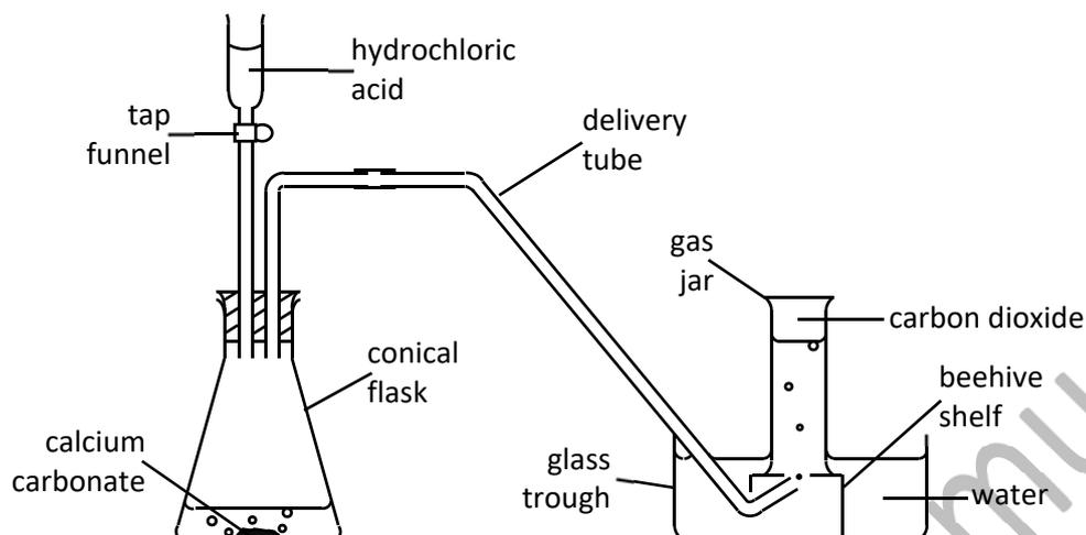
Carbon dioxide gas is prepared by adding a dilute acid like hydrochloric acid or nitric acid to a metal carbonate like calcium carbonate or sodium carbonate. Carbon dioxide is collected over water.
