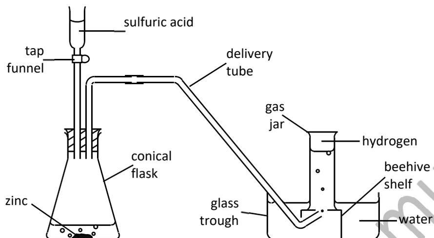
Hydrogen gas is prepared by adding a dilute acid like hydrochloric acid or sulphuric acid to a metal like magnesium or zinc. The hydrogen is collected over water.
