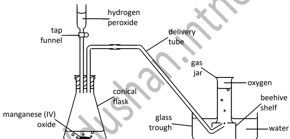
Oxygen gas is prepared by decomposing hydrogen peroxide faster using manganese (IV) oxide. Oxygen is collected over water.
